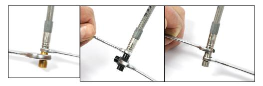
Choose a flat wrench which fits onto the connection. Place with an 8mm wrench at Hexagon on the threaded nipple and tighten the screw by **60°** (from tip to tip on a hex).
